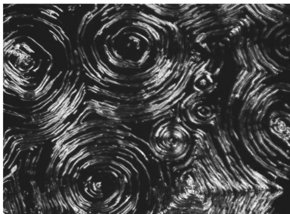
FIGURE 6 Microphotographs of UTGBC* phase at 80°C (235X).
